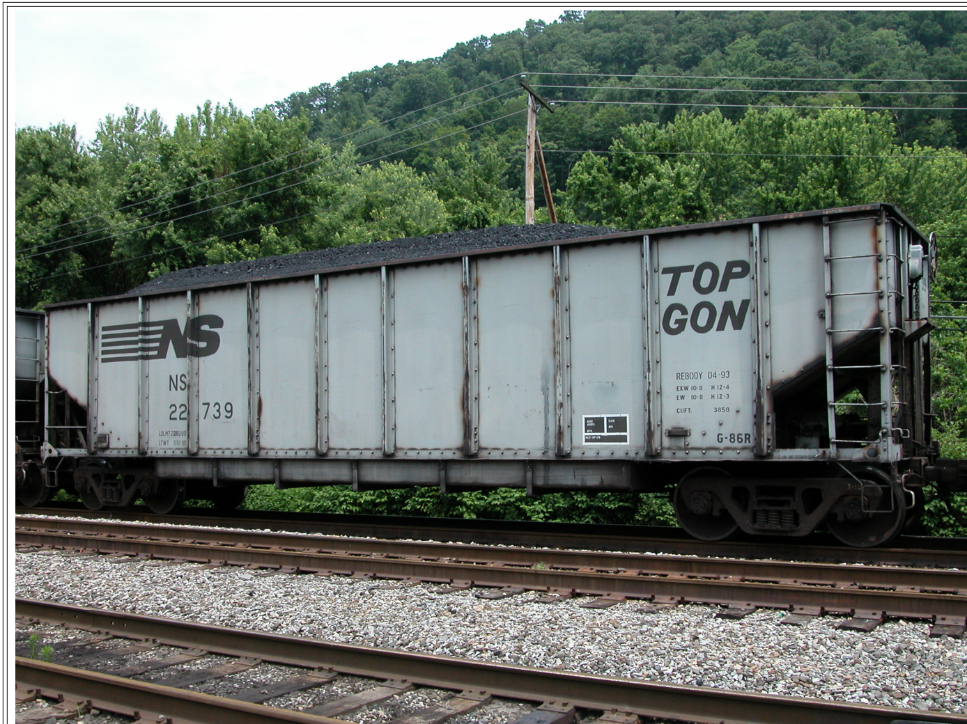
NS 22739 in Diamond, WV during 2005. The frame was originally built in 7-75. The car was rebodied in 4-93. Cubic foot capacity, 3850.
